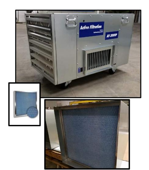
Active Filtration units can be adapted with a electrostatic washable pre-filter that can be used repeatedly in shops with a simple process of washing the filter. The reusability of the filters make it ideal for the shop with constant large particles like saw dust.
